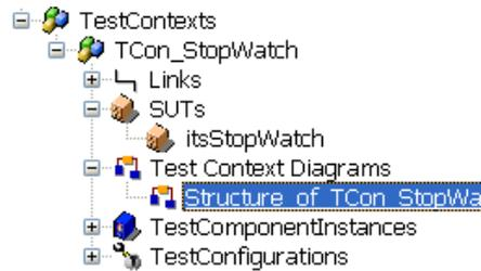
2 Have a look on the newly created Test Context Diagram „Structure\_of\_TCon\_StopWatch“, and view the resulting parts in the composite class „TCon\_StopWatch“ of our test context.
