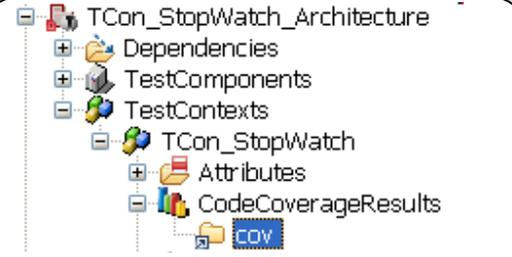
**3** After test case execution has finished, by double clicking the code coverage element in the browser you can open the code coverage report.
