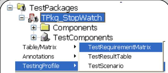
**1** Select the test package "TPkg\_StopWatch" and select "Add New -> TestingProfile -> TestRequirementMatrix".
