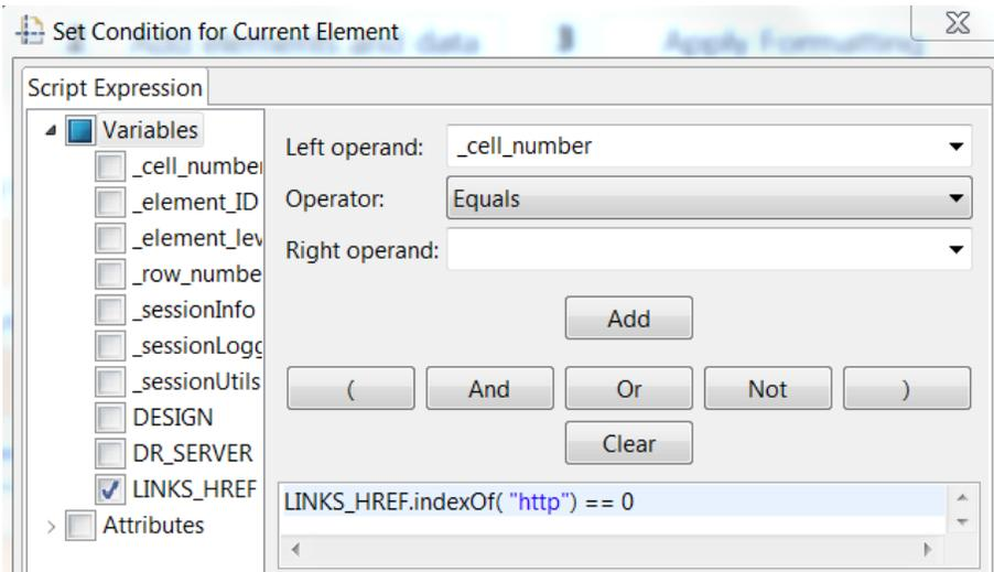
We utilize here the fact that for an element that does not have any links the Links element will not be present and hence the LINKS\_HREF variable will not be assigned a value by the container. If, on the other hand, there is at least one link, the LINKS\_HREF variable will be assigned the URL of the [Links API](#) which we expect should start with the string “http”.
