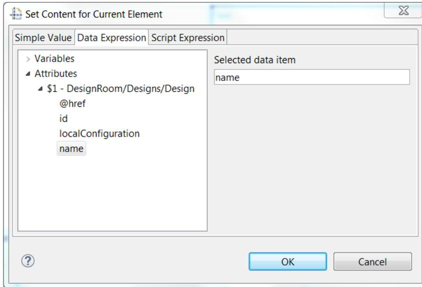
Alternatively you can drag the “name” attribute from the **Data Source** view and drop it onto the Text item.
