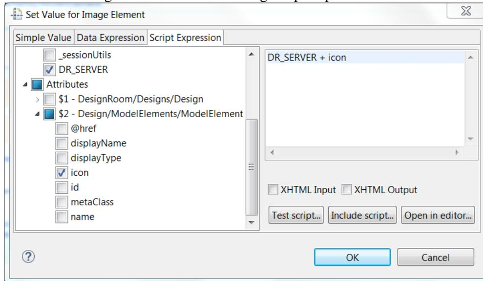
The `icon` attribute from the `ModelElement` element contains the path to the icon of the model element, so we just need to append that to the `DR_SERVER` variable to obtain the full URL of the icon.
