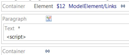
Note the icon on the paragraph that shows that it has an attached condition. It will only be included in the report for elements where the condition is fulfilled.
