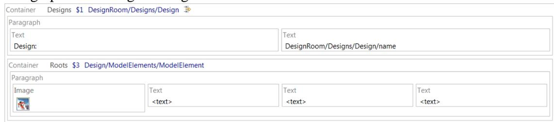
6. Contrary to the Designs data source, the Roots data source must be dynamic. That is, rather than configuring it once when generating the report, it must be configured once for each design (since the design is a parameter in the URL that is bound to this data source). To configure the Roots data source dynamically, place a Data Source Configuration item just before the Roots container:
