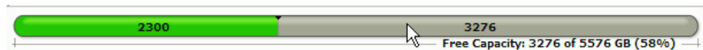
Figure 27. DS8000, Storwize, and SAN Volume Controller – Amount (GB) and percentage of free capacity on the storage pool
