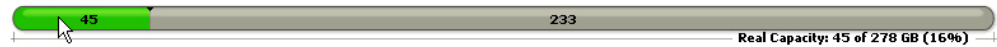
Figure 26. DS8000, Storwize, and SAN Volume Controller – Amount (GB) and percentage of real used capacity on the storage pool
