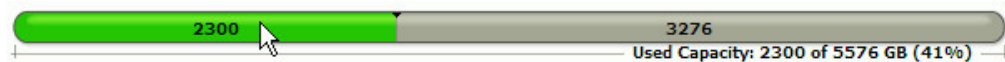
Figure 29. Storwize V7000 Unified and SONAS – Amount (GB) of used capacity on the storage pool or file system
