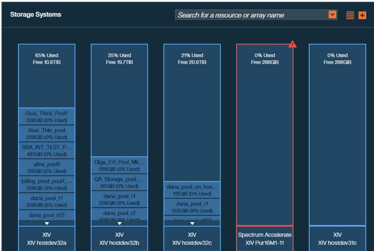
Figure 31. Storage Systems pane, bar view
