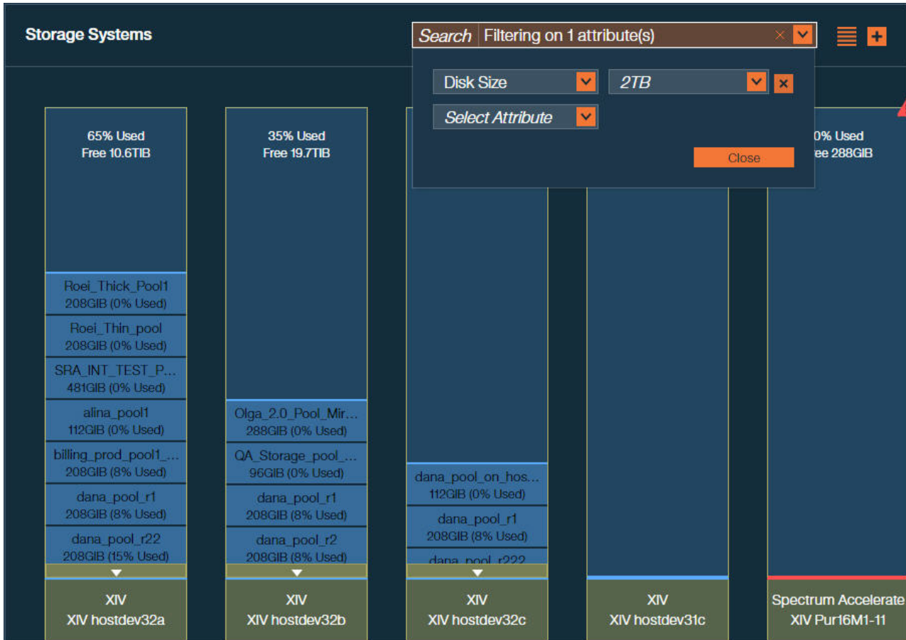
Figure 36. Storage Systems pane with storage elements filtered according to disk size
