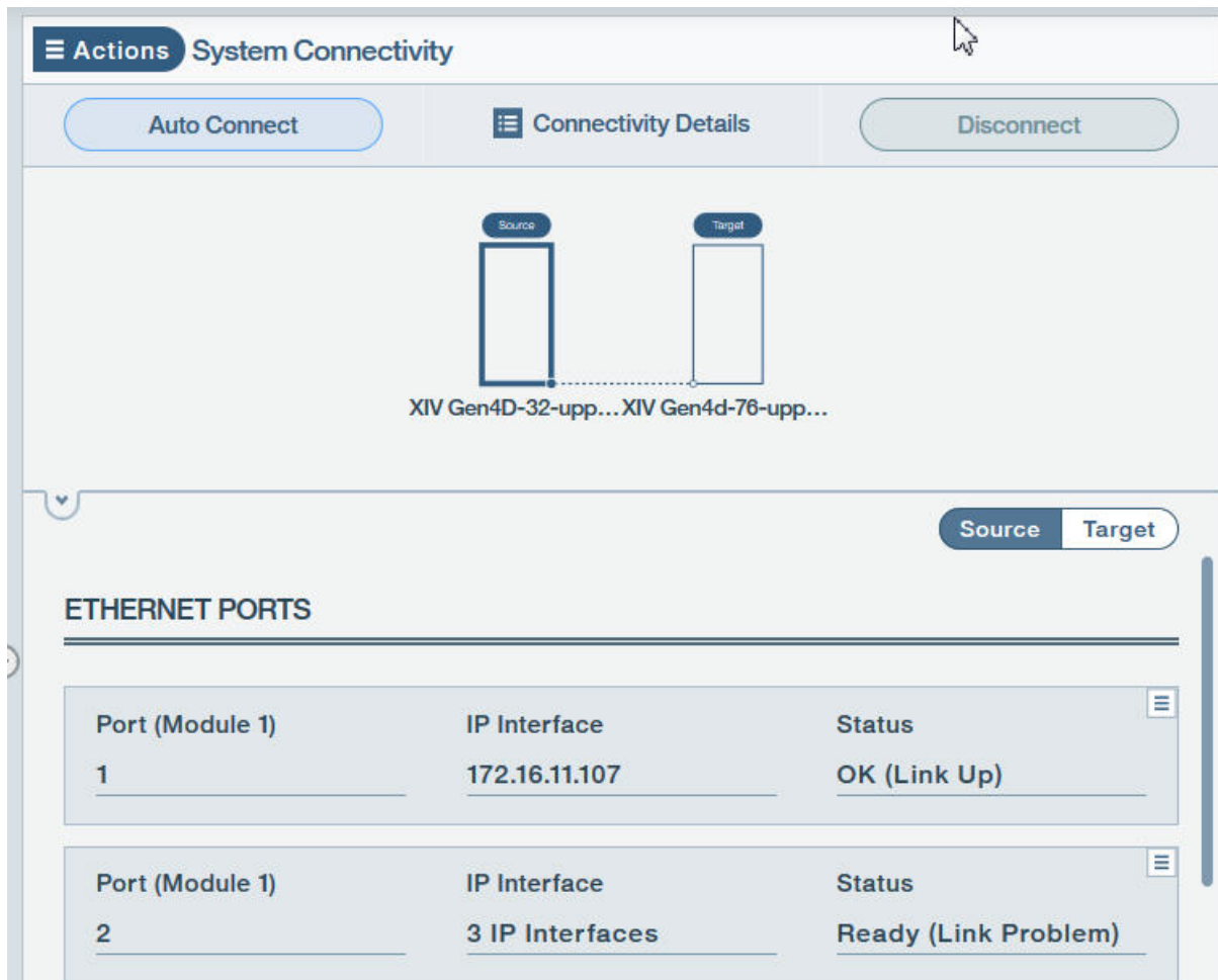
Figure 9. System Connectivity view
