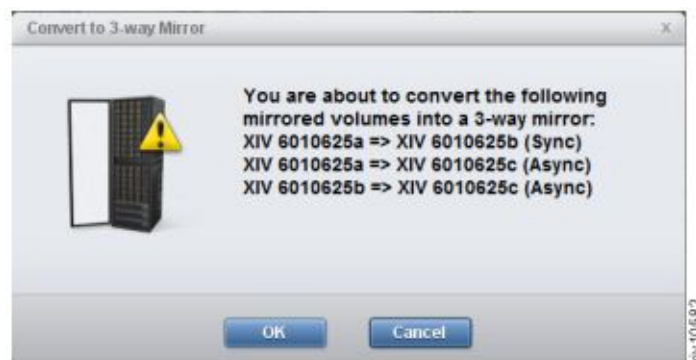
Figure 42. Converting to 3-way Mirror (when the mirror relation connectivity is in place)
