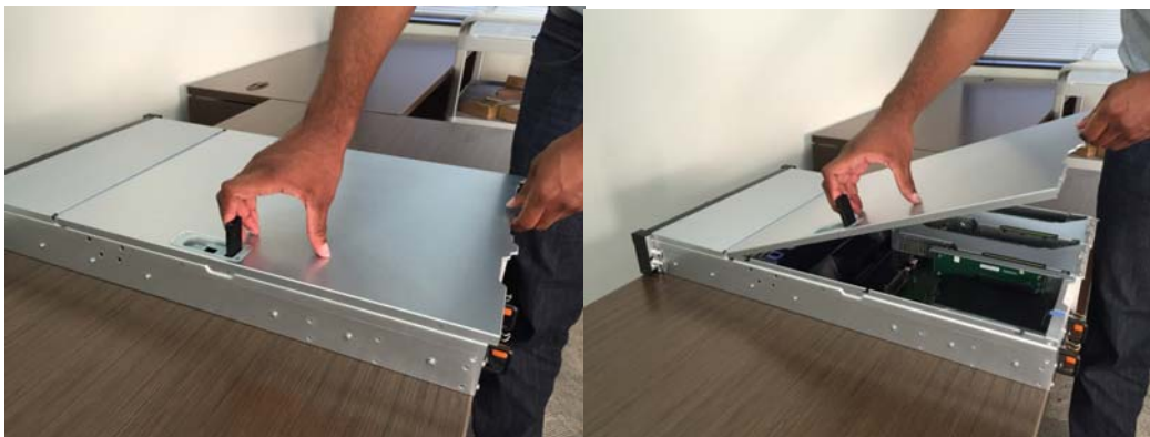
Figure 12. Removing the cover from the SV1
