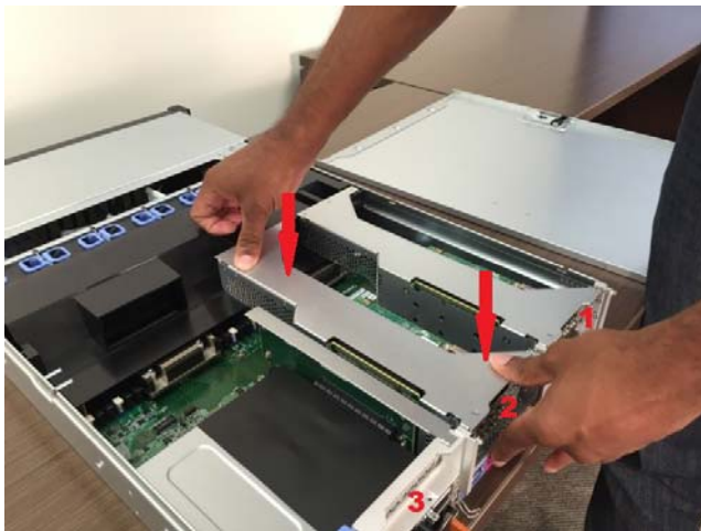
Figure 23. Replacing the SV1 PCI riser-card assemblies
