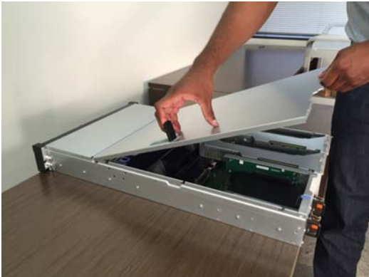
Figure 25. Replacing the SV1 cover
